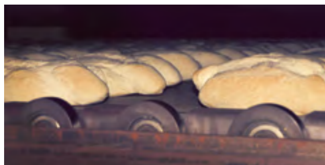
Baking oven chain with flanged roller and high temperature bearing (>600 F).
