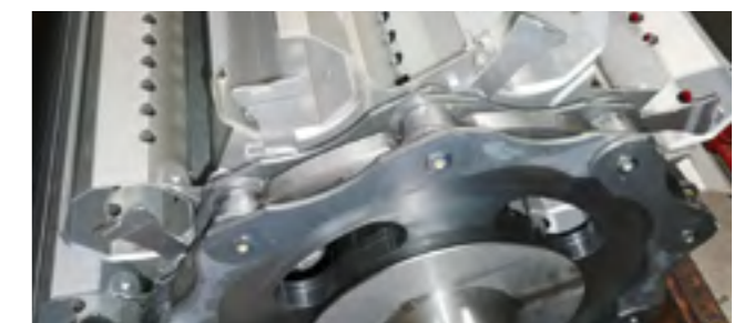
Stainless steel chain for sterilizing vegetables, frozen food, and pet food.
