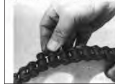
Chain clip installation method
